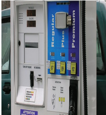
Transponder-based "smart" gas pump from Oregon's VMT pilot program (above) and typical receipt (above right) with itemized taxes/fees
