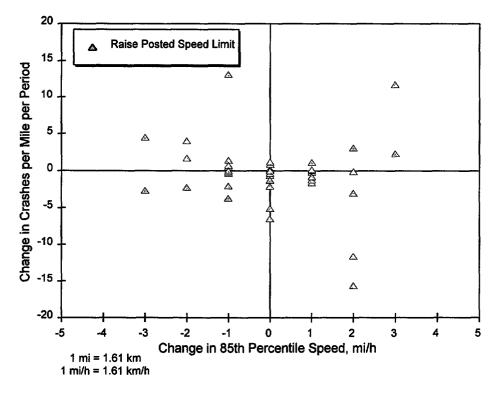
Figure 36. Before and after changes in crashes vs. changes in the 85th percentile speeds at sites where speed limits were raised.
