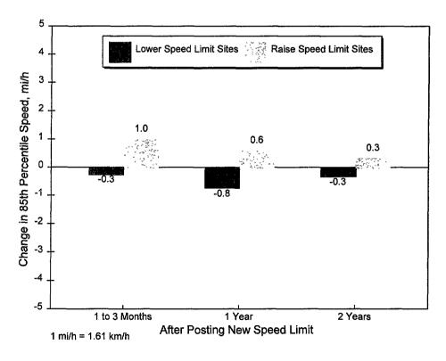
Figure 32. Mean changes in 85th percentile speeds at five sites where speed limits were lowered and at six sites where speed limits were raised.
