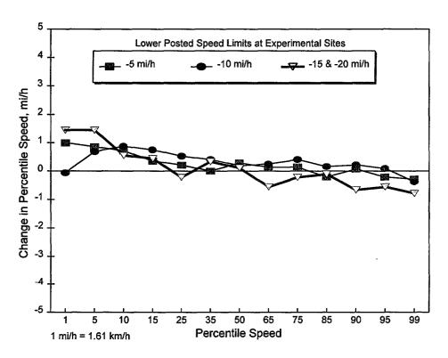
Figure 18. Before and after changes in percentile speeds at the comparison sites corresponding to the experimental sites where speed limits were lowered.
