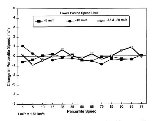
Figure 20. Net change (experimental minus comparison) in percentile speeds at sites where speed limits were lowered.
