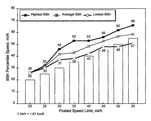
Figure 8. 85th percentile speed vs. posted speed limit for the comparison sites.
