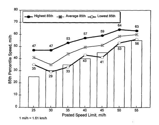
Figure 6. 85th percentile speed vs. posted speed limit for the experimental sites after the speed limits were altered.
