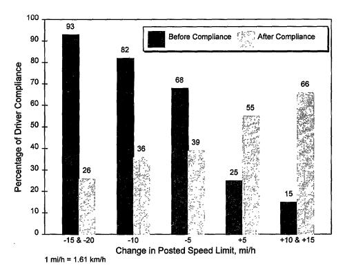
Figure 27. Driver compliance before and after speed limits were changed at the experimental sites.
