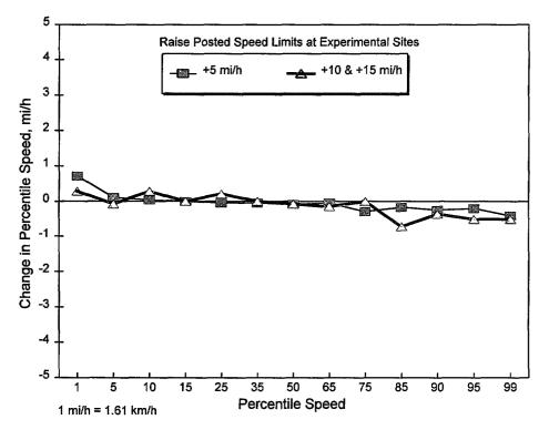
Figure 19. Before and after changes in percentile speeds at the comparison sites corresponding to the experimental sites where speed limits were raised.
