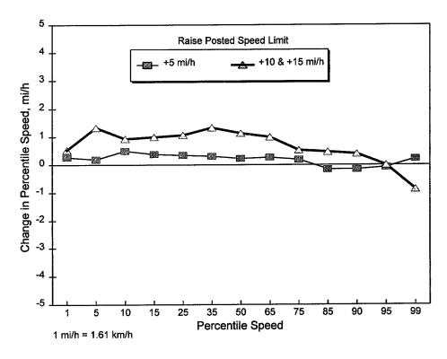
Figure 17. Before and after changes in percentile speeds at the experimental sites where speed limits were raised.
